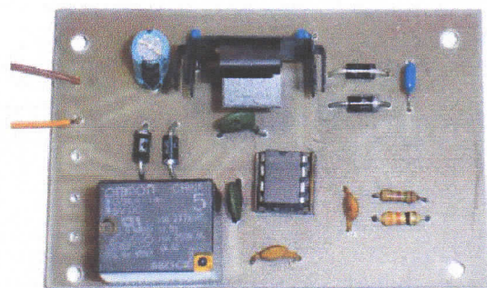
Figure 11 — Assembled upconverter board — ready for final assembly.
